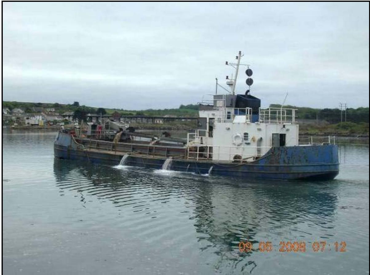
Alternative vessels may have reverse pumps but vessel size, both length and draft, will always be an issue within this dredged area. There are smaller vessels available but they would then face challenges in operating in the exposed channel and bar areas.
