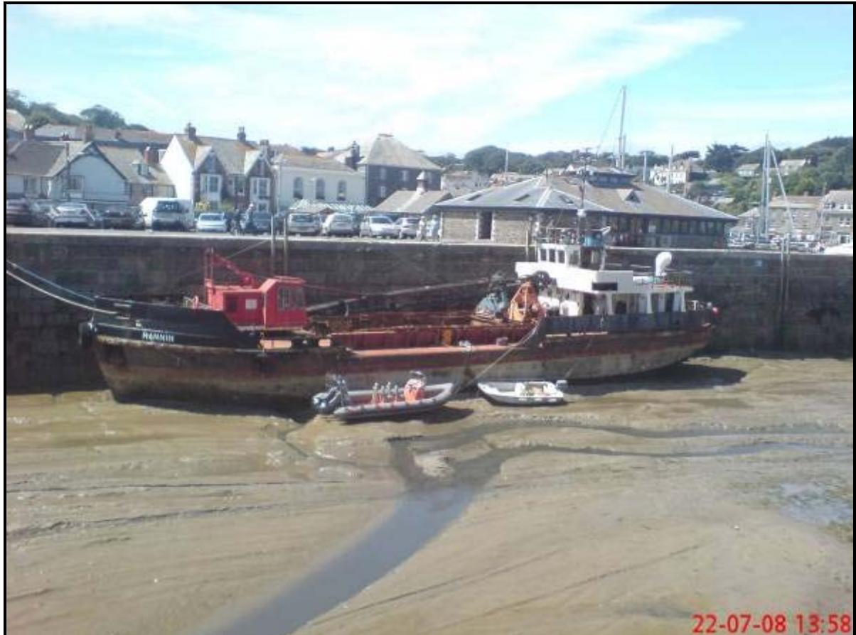
However, this type of dredger causes holes to be created which fill with seaweed and other materials. This was found to be an issue when re-introducing the cutter suction dredger to the same areas. Dredging rates are similar to the cutter suction dredger.
